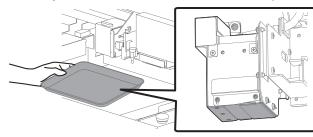
Use a paper towel to clean dust or ink off the underside of the UV-LED lamp.
