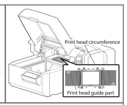
Use the cleaning stick to remove the ink and dust on the bottom of the carriage.
